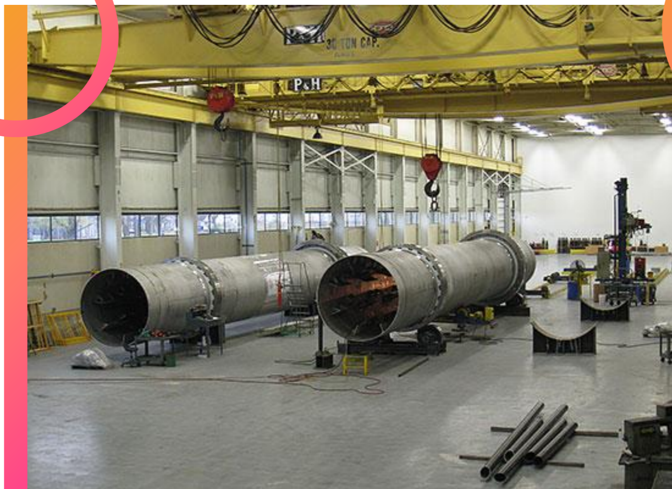
Jacketed Piping Fabrication
